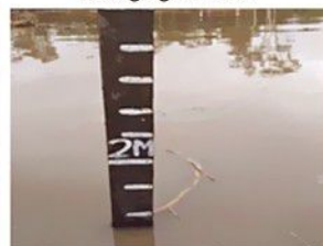
Tide Gauge for monitoring of the depth
